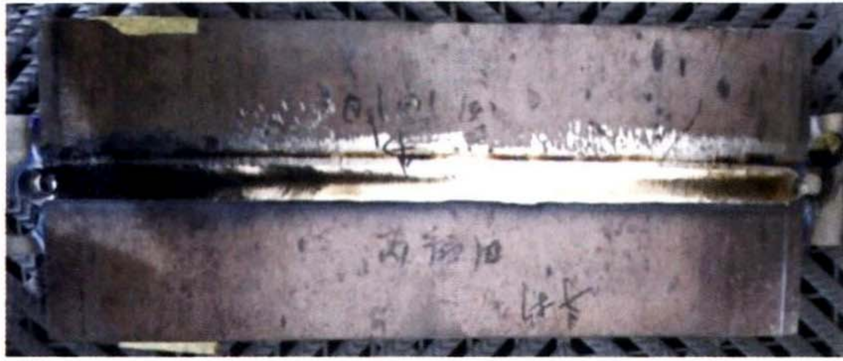
Fig. 4 Macroscopic morphology of the weld
